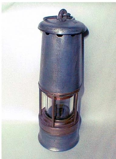
Coal miners used to work using an oil lamp for light. With the invention of the Davy lamp (pictured on the left) in 1815, there was far less risk of methane catching alight in the mine.
